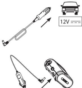
Insert the plug of the cable into the 12V DC cigarette lighter socket of the car/camper/boat. Check the vehicle's operating manual to ensure that the voltage supplied is 12Vdc.
