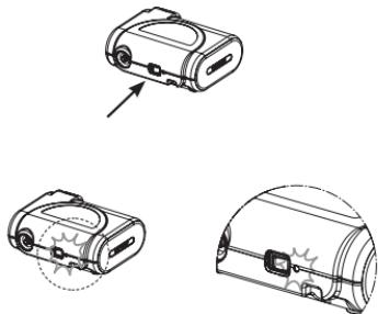
Make sure the switch is OFF, in position ( 0 ).
