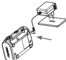
Insert the "L" plug of the power supply cable into the DC plug of the device.
