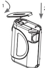
Attach the “**AIR FILTER**” cover 1 to the unit by hooking it into the front of the housing and 2 by pressing the back down until it snaps into place.
