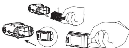
Before inserting the battery, remove the sponge/muffler from the battery compartment. Insert the original Flaem battery, which you can obtain from your dealer.
