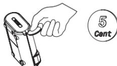
To remove the "BATTERY" cover, pry it off with a small coin of appropriate size by inserting it into the rear slot.
