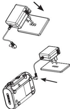
Plug the power supply unit into the mains socket, checking that it is not difficult to disconnect from the mains.
