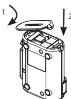
Attach the "BATTERY" cover 1 to the appliance by hooking it into the front of the housing 2 and pressing the back fully down until it snaps into place.
