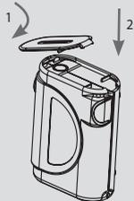
Replace the "AIR FILTER" cover by 1 positioning the front part in the seat and 2 gently pressing on the rear part until it snaps securely into place.
