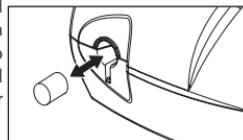
The filter is designed so that it is always fitted in its housing. Do not replace the filter during use. Only use original Flaem accessories or spare parts, no liability is accepted if non-original parts or accessories are used.
