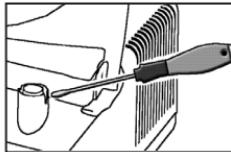
**To replace the filter, pull it out as shown in the figure.**
