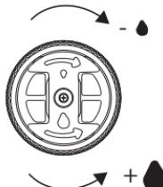
To use the bowl without selector, firmly grasp the bowl body and use your other hand to rotate the particle size regulator (B2.4) clockwise until it is ejected from the upper part (B2.3).
